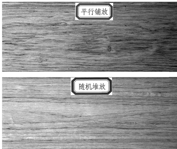
图4 不同铺装方式对重组木纹理的影响 Fig.4 Textures of scrimbers made by different forming methods
